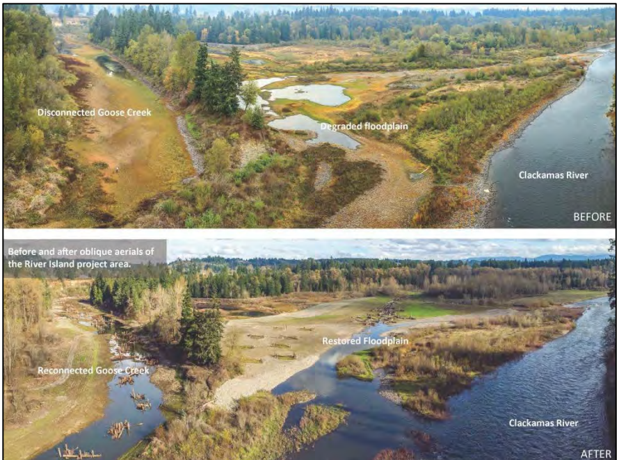
Metro’s River Island Natural Area before (top photo) and after (bottom photo) restoration. Years of gravel mining and record flooding in 1996 altered the area’s landscape and changed the Clackamas River’s path. Restoration is improving floodplain vegetation and function and creating sustainable habitats. Source: Brian Vaughn, Metro
